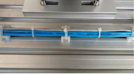
A photograph showing blue cables and black hoses bundled together on an aluminum profile. Both are held by white plastic clips, which is an incorrect practice. |
